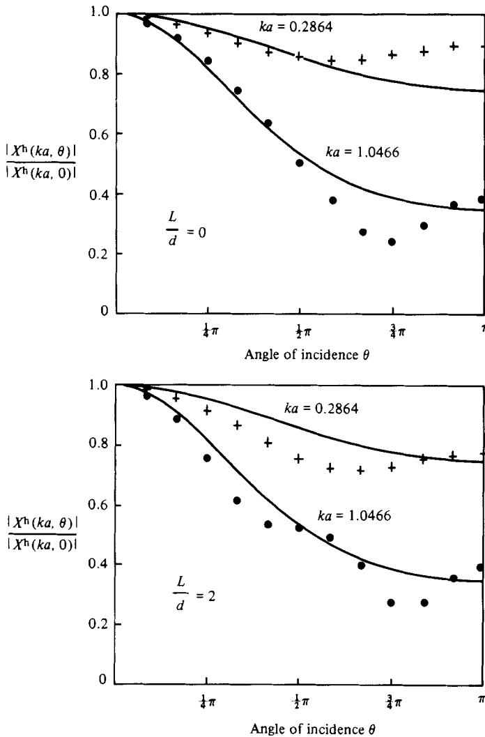
FIGURE 6. Comparison of the angular dependence of the exciting-force amplitude using the approximate theory (solid lines) and numerical calculations (●, +) for  $ka = 0.2864, 1.0466$  and  $L/d = 0, 2$ .
