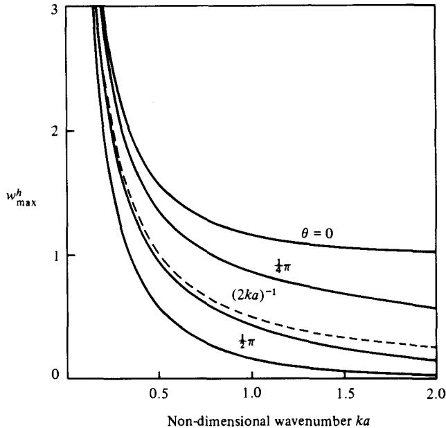
FIGURE 2. The maximum capture-width ratio for a harbour system for various angles of incidence in comparison with the result  $(2ka)^{-1}$  for a heaving axisymmetric structure.
