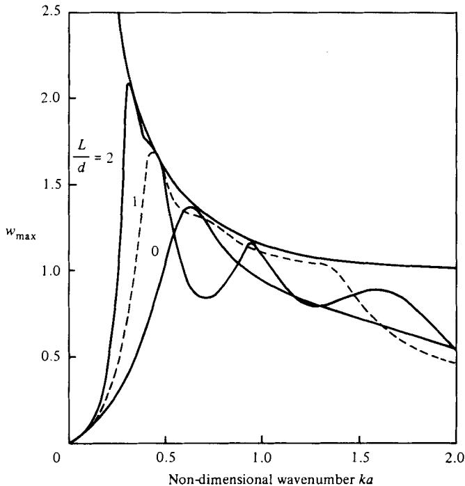
FIGURE 7. The capture-width ratio for  $L/d = 0, 1, 2$  using an optimized (real) damping constant  $A$  compared with  $W_{\max}^h$  for normally incident waves ( $\theta = 0$ ).
